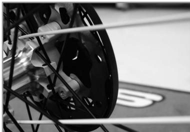
Wear on the thickness of discs occurs in the contact zone between the disc and the brake pads.
