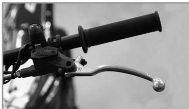
The clutch lever is on the left grip of the handlebar. To adjust the clutch lever's position, use the adjustment screw intended for this purpose (📖p. 70).
