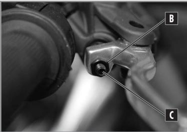
To properly press on the clutch while shifting, it is essential that the position be adapted to the driver.
