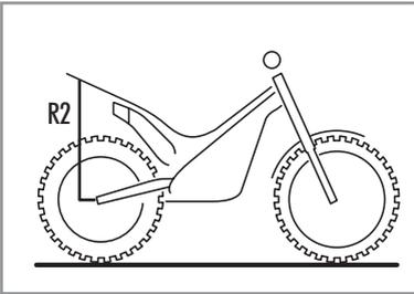
$R1 - R2 = \text{Static shock absorber sag.}$
