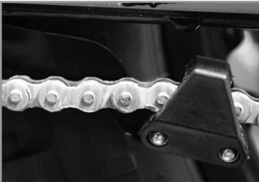
The chain tensioner is one of the most-ordered elements, especially the spring, which is responsible for keeping pressure on the chain.
