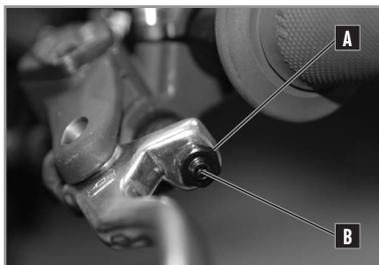
Adjust the tension of the clutch handle with the threaded rod **B**.
