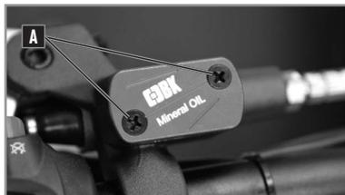
The clutch fluid tank is above the handle.
